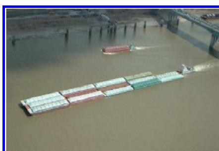
One or more non-powered IWT vessels which are towed or pushed by one or more powered IWT vessels.
