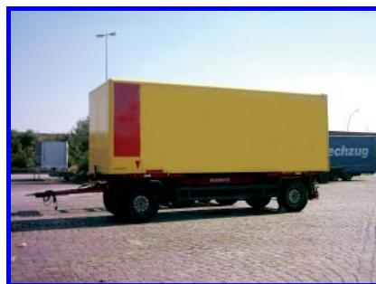
Goods road vehicle designed to be hauled by a road motor vehicle.
