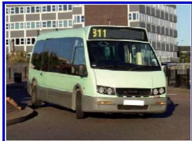
Passenger road motor vehicle designed to carry 10- 23 seated or standing persons (including the driver).
