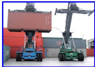
Tractor vehicle with front equipment for lifting, stacking or moving ITUs.
