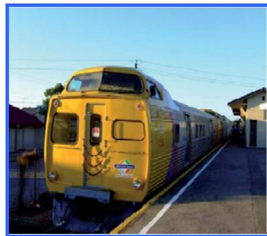
Tractive railway vehicle with motor constructed for the conveyance of passengers or goods by rail. *The definition of the various categories of locomotives (electric, diesel) apply, mutatis mutandis, to railcars.*
