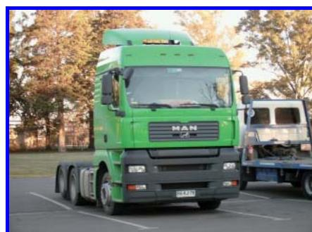
Road motor vehicle designed, exclusively or primarily, to haul other road vehicles which are not power-driven (mainly semi-trailers).
