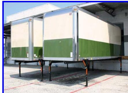
A freight-carrying unit optimised to road vehicle dimensions and fitted with handling devices for transfer between modes, usually road/rail.
