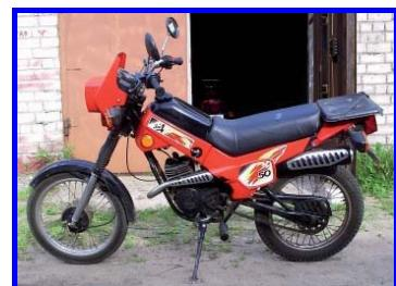
Two, three or four-wheeled road motor vehicle which is fitted with an engine having a cylinder capacity of less than 50cc (3.05 cu.in) and a maximum authorized design speed in accordance with national regulations.
