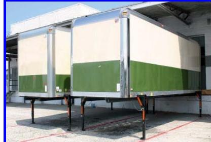
A freight-carrying unit optimised to road vehicle dimensions and fitted with handling devices for transfer between modes, usually road/rail.
