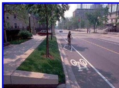
Part of a carriageway designated for cycles and distinguished from the rest of the carriageway by longitudinal road markings.
