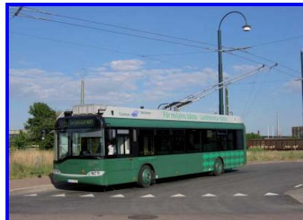
Passenger road vehicle designed to seat more than nine persons (including the driver), which is connected to electric conductors and which is not rail-borne.
