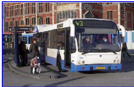
Passenger road motor vehicle designed to carry more than 24 persons (including the driver), and with provision to carry seated as well as standing passengers.
