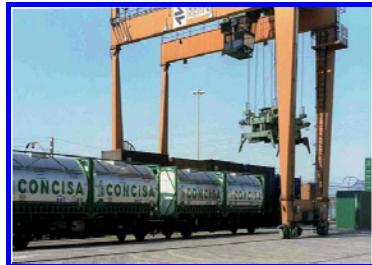
A rubber-tyred overhead lifting vehicle for moving or stacking containers on a level reinforced surface.
