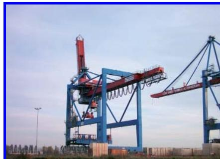
An overhead crane comprising a horizontal gantry mounted on legs, which are either fixed, run in fixed tracks or on rubber tyres with relatively limited manoeuvre. The load can be moved horizontally, vertically and sideways.
