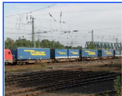
Wagon specially built or equipped for the transport of intermodal transport units (ITUs) or other goods road vehicles.
