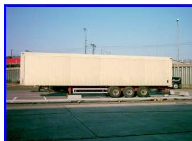
Goods road vehicle with no front axle designed in such way that part of the vehicle and a substantial part of its loaded weight rests on the road tractor.
