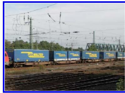
Wagon specially built or equipped for the transport of intermodal transport units (ITUs) or other goods road vehicles.
