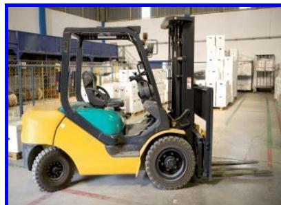
Vehicle equipped with power-driven horizontal forks, which allow it to lift, move or stack pallets, containers or swap bodies. The latter two are usually empty.
