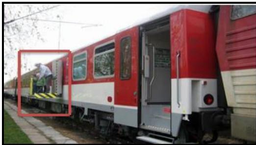
**Figure5** Bdgsheer wagon with a hydraulic lifting platform
