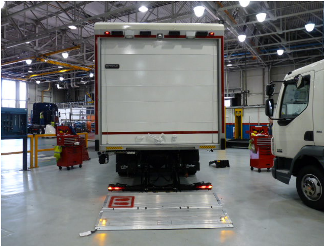
Figure 2: Operating (fixed) position for tail lift (vehicle parked)
