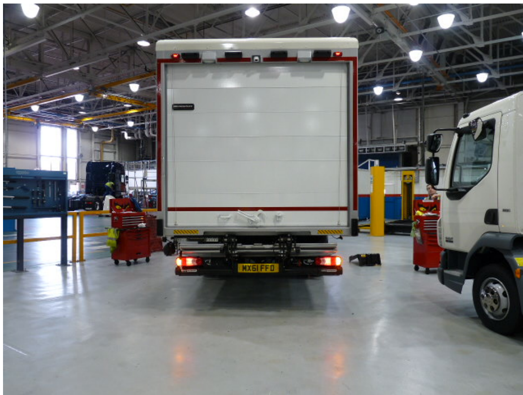
Figure 1: Normal position of use for vehicle (tail lift stowed)
