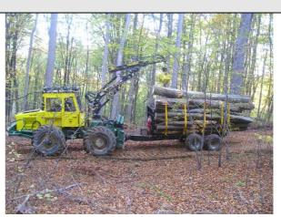
Aforementioned vehicle corresponds to the definition of the wheeled tractor of category T according the directive 2003/37/EC.
