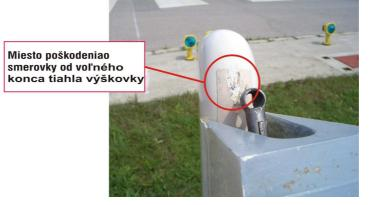
From the state of damage to the vertical rudder it results that the damage was caused by movement of the loose end of the elevator rod.
