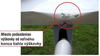
The state of damage to the elevator also leads to the conclusion that the damage was caused by the loose end of the elevator rod.
