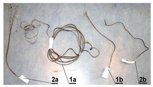
In case of all examined parts of the steel rope the type conformity was demonstrated, i. e. in all these parts belonged to a rope with the same construction and the same dimensions – all parts of the rope had a diameter of 8 mm and diameters of all wires lied within a range of, 0.48 to 0.50 mm. Moreover, all parts of the rope showed a regular right-hand lay
