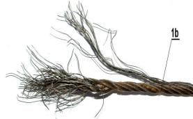
The damaged end of part of the rope submitted as evidence No. 2b again showed signs of forceful rope twisting.
