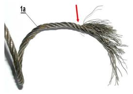
From the mechanism of damage to this part of rope with a marked twisting component it can be concluded that it was connected to a partially untwisted end of rope No.1b, found from the front section of the helicopter, which fully corresponds to the fact that if we damage the rope with marked twisting component by loading it, a higher rate of winding of rope strands will be observed on one side of the damaged area and untwisting of rope strands on the other side.
