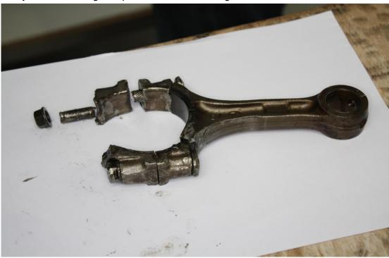
The loose connecting rod bumped into piston No. 4 until it completely destroyed it and pierced the engine block, thus making it unfunctional.
