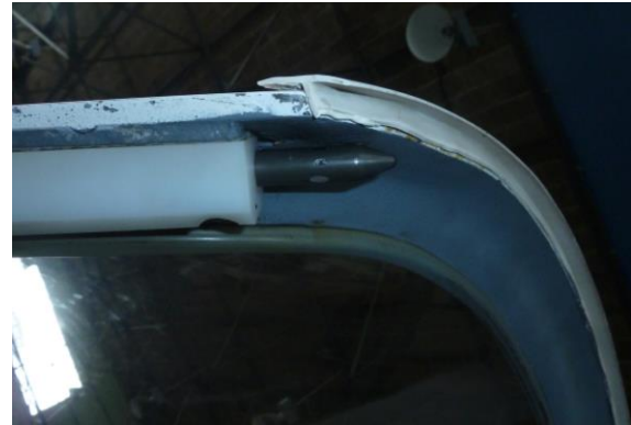
Fig.2 Detail of engaged locking wedge in the opened position
