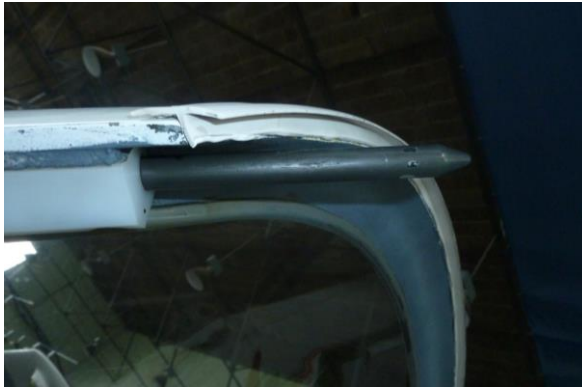
Fig.1 Detail of disengaged locking wedge in the closed position
