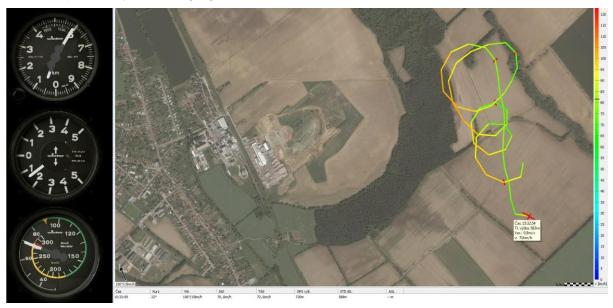
Subsequently the pilot commenced descent at course 300° with opened air brakes, intending to line up the landing axis of RWY14 by a left-hand turn. Following the lining up, according to the pilot's statement, he was unable to keep the landing direction, because the glider was continuously turning left. The pilot closed the air brakes and intended to continue the landing manoeuvre by lining up the axis of RWY 14 again in order to complete the left-hand turn.
