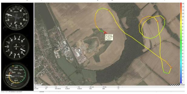
After the stopping of spin rotation the glider was in a steep dive low above the ground. Therefore the pilot decided to solve the situation by field landing in the direction of the glider, but all he managed to do was open the air brakes. Afterwards, the glider came into a harder slipping contact with the ground, which caused its damage. Further damage to the glider occurred in the ground roll phase, because it continued to turn left. The pilot left the damaged glider with help of a passer-by.
