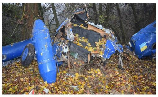
Fig.3 Rear part of the airframe with the right wheel of main landing gear and secondary fuel tank
