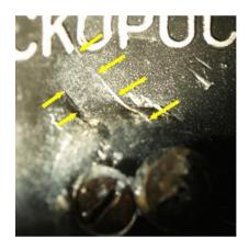
Fig.14 Detailed view of indents from edges of the broken part of the pointer
