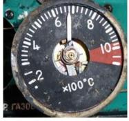
Fig. 12 Temperature of exhaust gases (left-hand engine)
