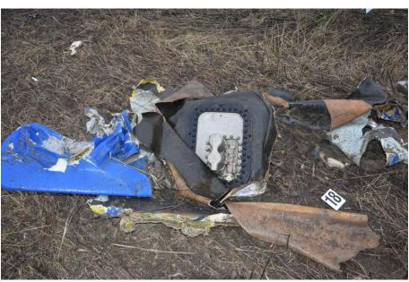
Fig. 10 Destructioned main fuel tank
