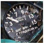
Fig.11 Lift rotor blade pitch
