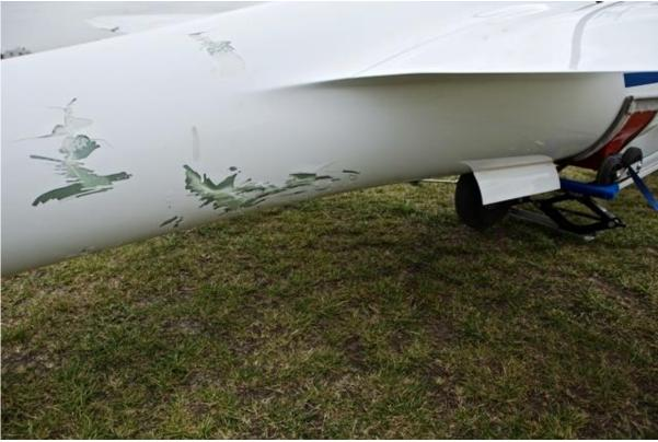
fuselage damaged in the centre-wing section.
