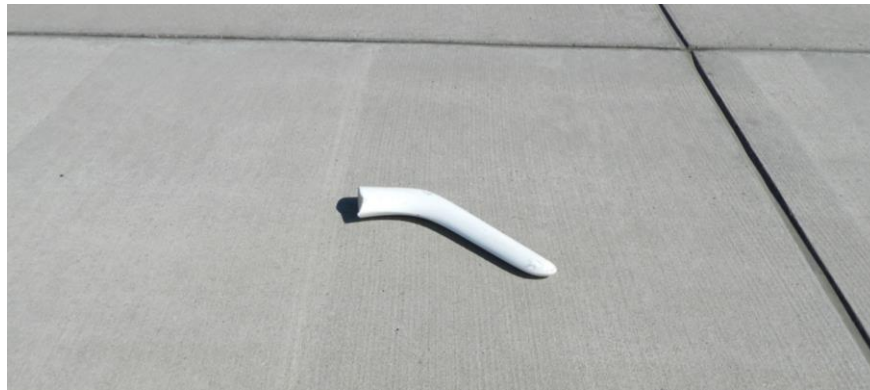
Part of broken radio antenna equipment
