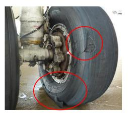
Picture 12 Detail of a damaged tyre
