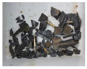
Picture 11 Fragments of landing gear components found on the RWY
