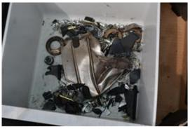
Picture 10 Fragments of landing gear components found on the RWY
