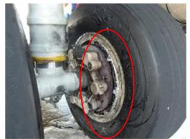
Picture 8 Details of the damage to the main landing gear
