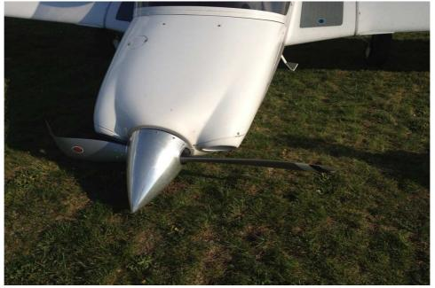
Damage to propeller and engine caused by violent stoppage when the propellertouched the ground.
