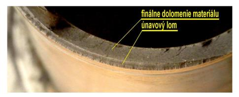
Fig. 4a Smaller opposite part of fatigue fracture and bevelled area of final material rupture
