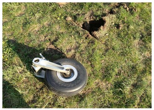
Breakage of fork and wheel of the front landing-gear
