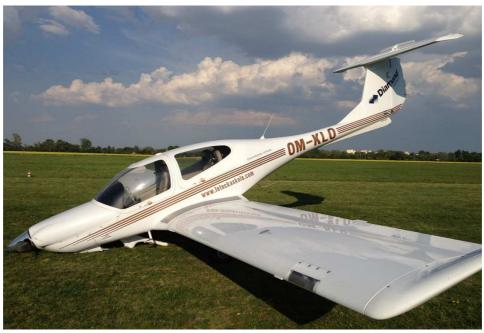
Breakage of the front landing-gear leg, damage to propeller and engine of aircraft
