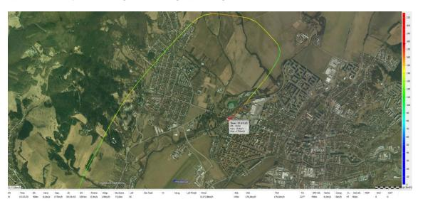
Approximately 50 m before the threshold of VPD22, at an altitude of 20 m, the pilot's landing speed was 214 km/h.
