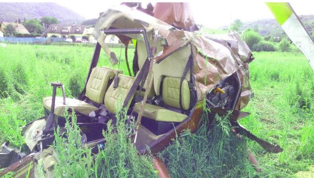
The fuselage was quite distorted and its front part was completely destroyed. Traces of earth were found on the wreckage of the fuselage, including the cylinder head of the main rotor and blades, so after the R44 hit the ground, it turned over on the front and the right side and the rotation was stopped by the skids.
