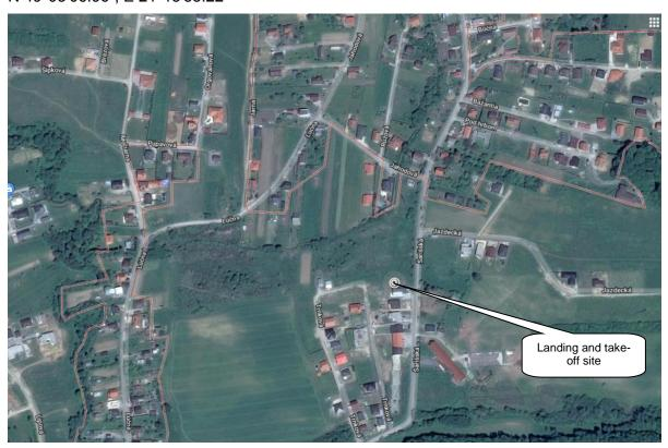
The landing and take-off site may be described as a 25x10 m area with a moderate incline, oriented in the direction 085°/265°, located near a family house with numerous obstacles in the surroundings. After landing, the R44 sat with its front part against the slope.
