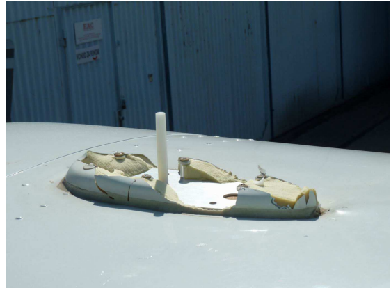
Damage to dorsal fin fairing
