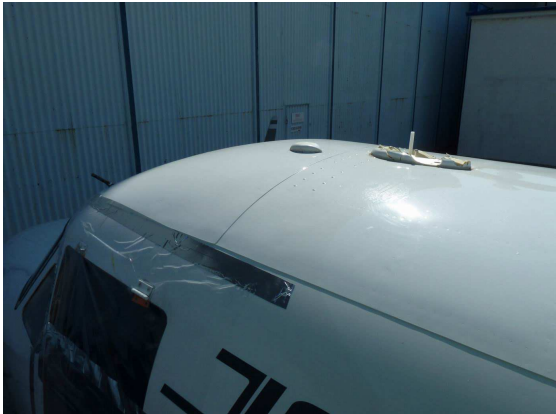
Damage Tail De-Ice boot vertical fin
