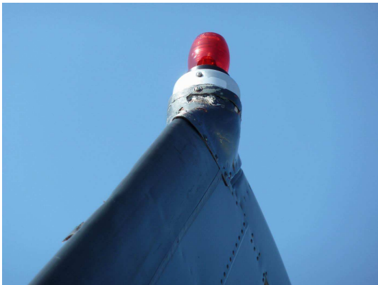
Damage Tail De-Ice boot vertical fin
