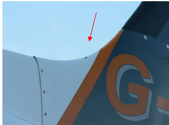
Damage to dorsal fin fairing
