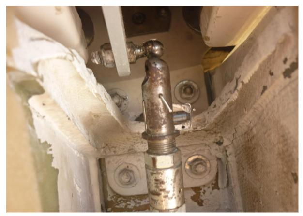
Picture 7 Unconnected elevator rod
