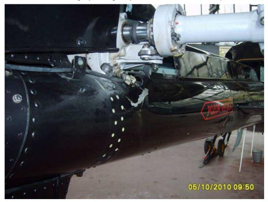
The anti-torque rotor of the helicopter was damaged and will have to be replaced.
