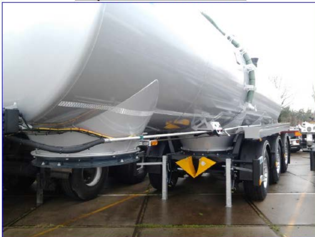
Lateral protection attached to the turntable of a steered axle
