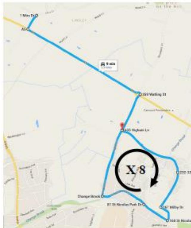
We have been approached by a technical service to allow the urban part of the RDE test to be carried out on a route around a residential area where they drive the same loop 8 times. The proposed route does meet all of the trip requirements and includes artificial stops to replicate urban traffic and meet the idle time requirement.
