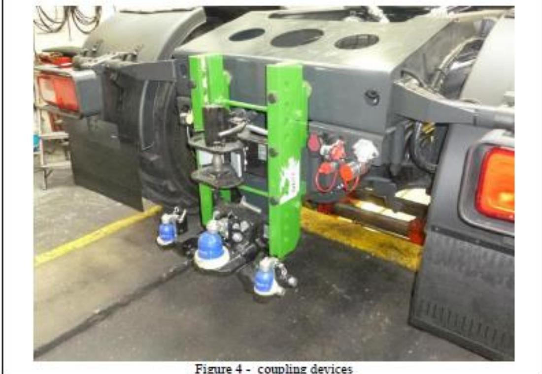
Figure 4 - coupling devices
