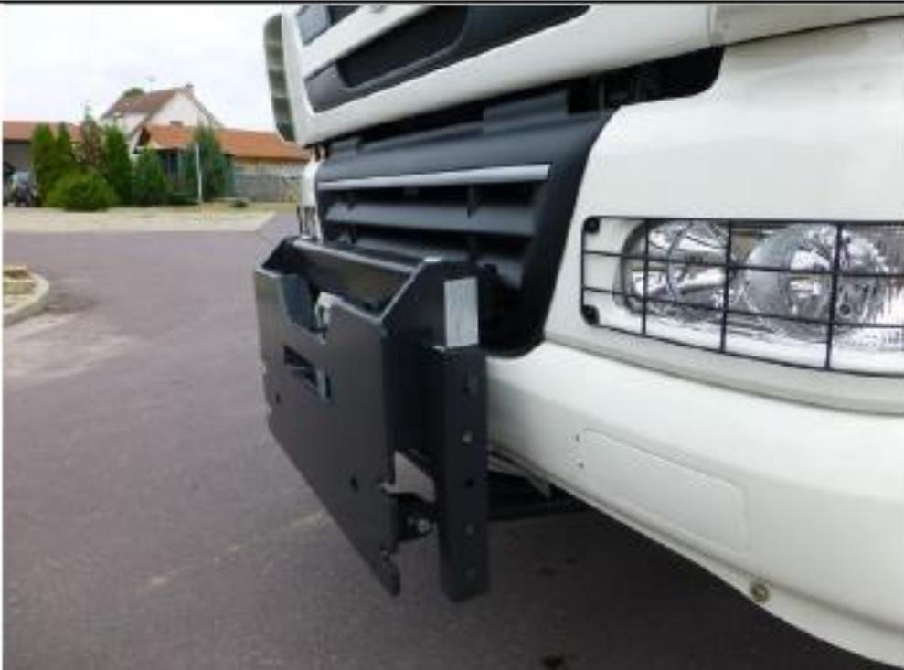
Figure 5 - front fixing plate, protection of the running light
